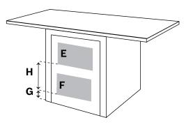
If the front of the appliance is covered, ventilation openings must be installed as shown and front/rear clearances adhered to according to closet installations. (see spec sheet)
